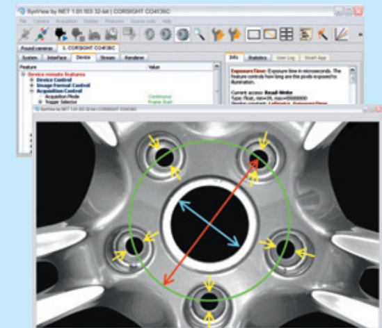
smart assembly: localisation > pattern recognition > data transfer to robot
